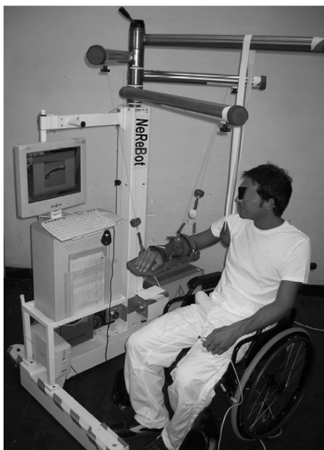
Fig 1. The patient's right forearm is fastened into the splint to receive sensorimotor stimulation with NeReBot (A) at the bedside and (B) in the sitting position.
