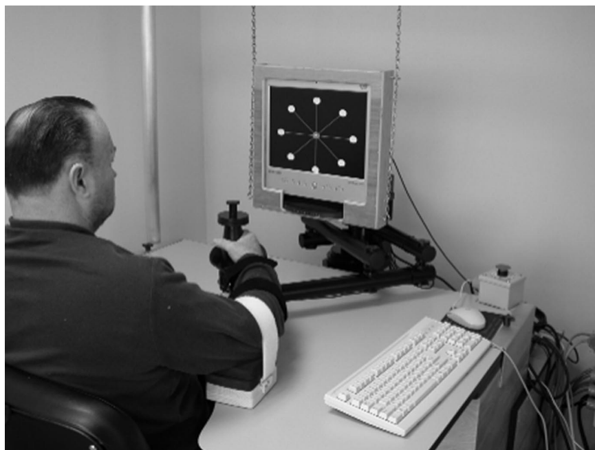
Figure 1: InMotion2 robot: a subject is shown performing robot-aided exercises. A cursor on the display corresponds to the position of the hand, and each target is highlighted sequentially as a goal for the subject to reach toward.
