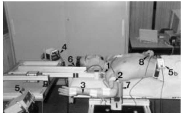
FIGURE 2. The experimental set-up, showing the position of the subject, the load cell (1), the electrogoniometer at the elbow (2), the electrogoniometer at the wrist (3 [not used in this experiment]), the amplifier and digital display of the load cell (4), the base unit (5a) and patient unit (5b) for the electrogoniometers, the head restraint (6), the armrest (7), and a hand-held switch (8 [not used in this experiment]).
