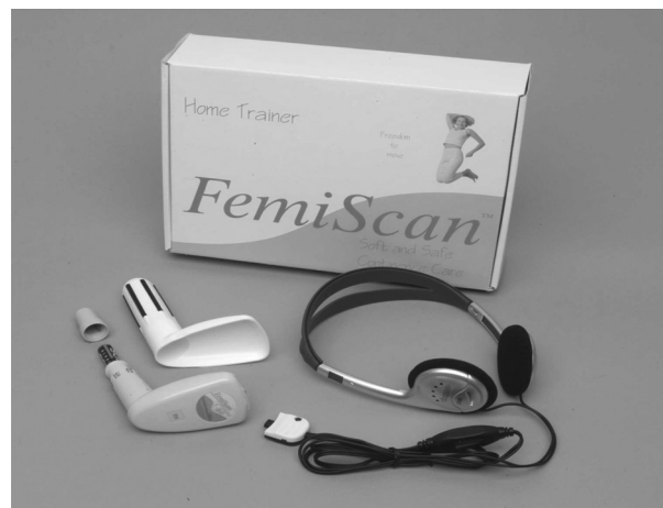
Fig. 1. A personal EMG-assisted biofeedback device (FemiScan TM , MegaElectronics, Kuopio, Finland) that contains an internal microprocessor capable of collecting training performed at home. Patient hears instructions for pelvic floor training by headphones.
